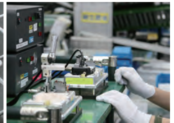
Air Leak Test
